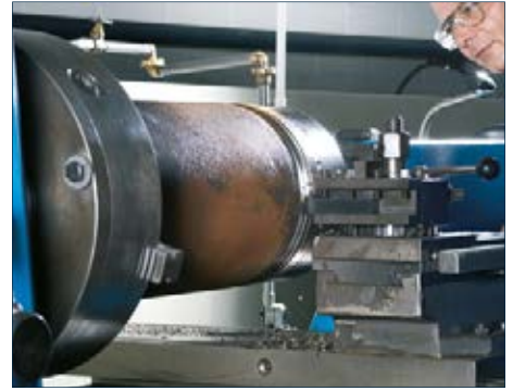
Reconditioning of a cylinder liner
