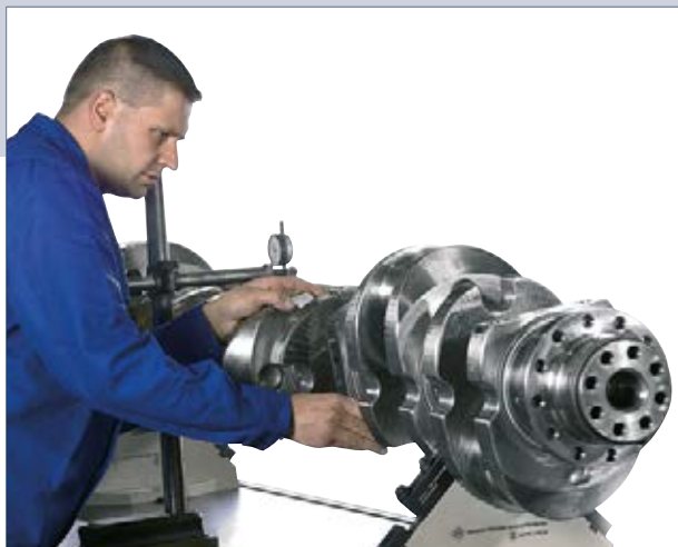
Run out inspection of a crankshaft
