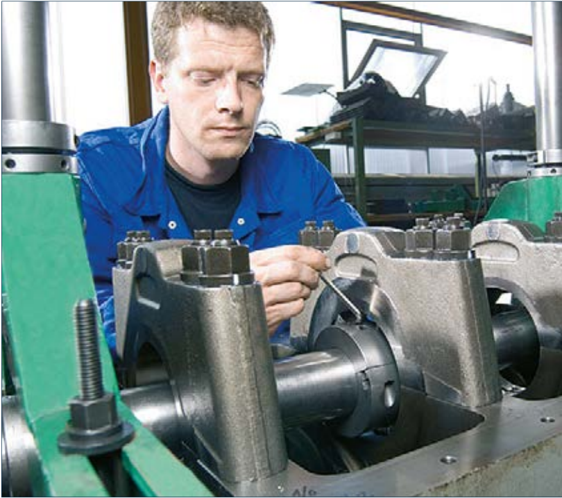
Boring of a main bearing base
